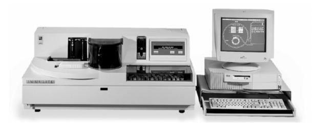
The Siemens DCP IMMULITE Automated Immunoassay System is a continuous, random access instrument that performs automated chemiluminescent immunoassays.
